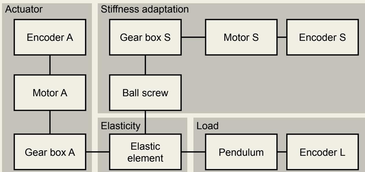
FIGURE 6: Reduced functional and structure graph of the VTS actuator. Edges indicate moving connections of the drive train elements. The housing is excluded
