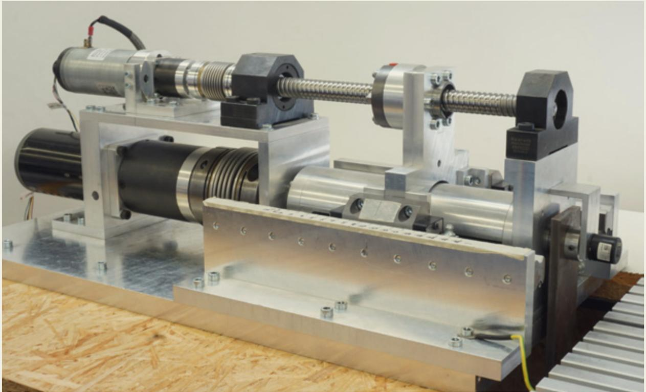
FIGURE 5: Variable torsion stiffness actuator
